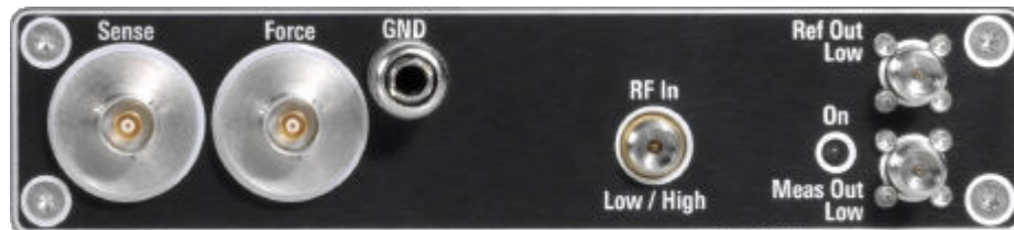
Figure 3-17: Connector panel of R&S ZVA-ZD110 Var 18
