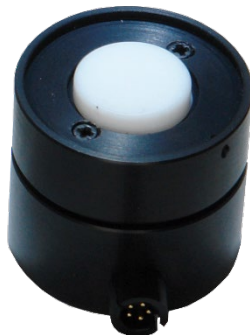
Fig. 3.10.31 Irradiance measuring head FLA 623 GS
