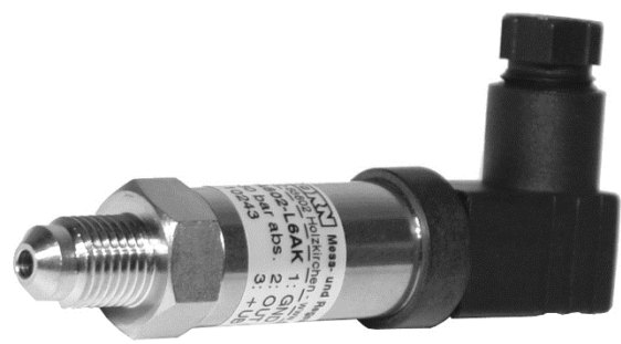
Fig. 3.8.4 Type FD A602LxAK: Standard version with 7/16" external thread, membrane inside
