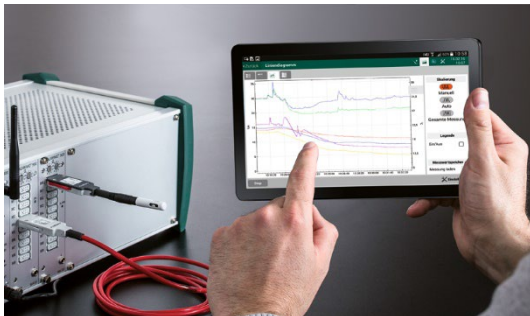
Fig. 2.5 Tablet with app for ALMEMO® 500
