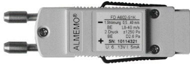
Fig. 3.8.7 Pressure measuring connector for differential pressure FD A602 S1K
