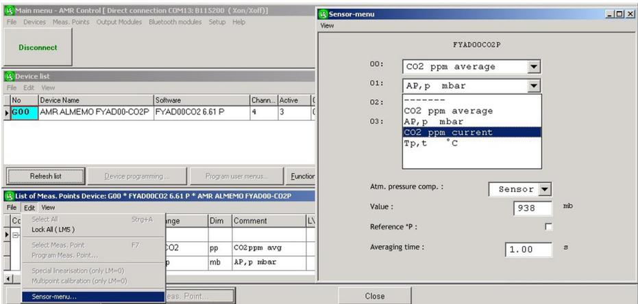
Initially the ranges for the measuring channels can be configured from a list (\* factory default settings).
