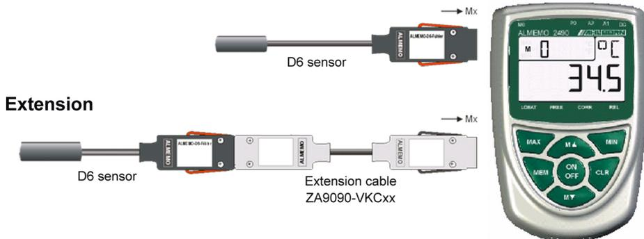
The operating radius of these sensors when connected to a measuring instrument can be extended by means of universal extension cables ZA9090-VKCxx; measured values and connector programming can then be transmitted interference-free in serial form via an RS485 driver.
