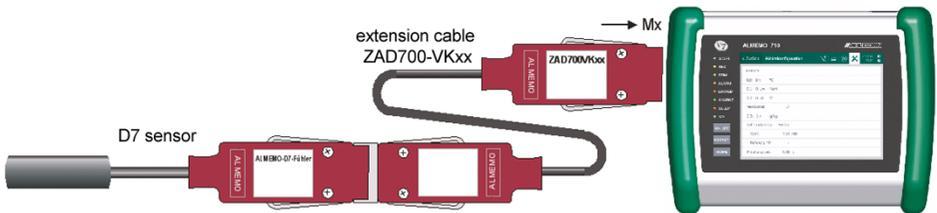
The operating radius of these sensors when connected to a measuring instrument can be extended by means of extension cable ZAD700-VKxx; measured values and connector programming can then be transmitted interference-free in serial form via an RS-422 driver. For electrical isolation adapter cable ZAD700-GT can be used.
