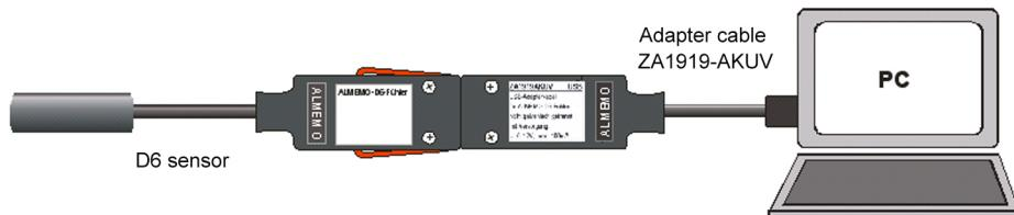
The ALMEMO® D6 sensor can be connected directly to a PC using USB adapter cable ZA1919-AKUV at a baud rate of 115.2 kilobaud. A microcontroller incorporated in the adapter cable automatically sets the power supply, baud rate, and device address that the sensor requires.
