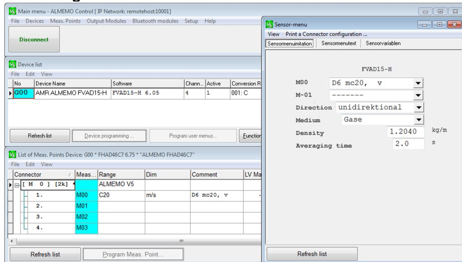
Depending on the type of rotating vane, initially only 1 measuring range is programmed (\* factory default setting). If needed, this range can be changed, and on the 4 measuring channels additional ranges such as frequency or revolutions per minute can be configured (see table below).
