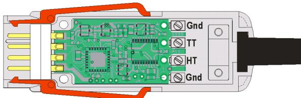
With hand-held psychrometer FNAD846 the sensors are soldered to the plug circuitry and thus powered via the ALMEMO® device.
