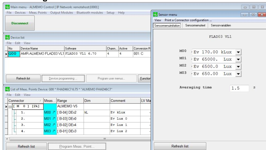
The measuring ranges of the measuring channels can be configured according to a list of ranges (\*factory default settings):
