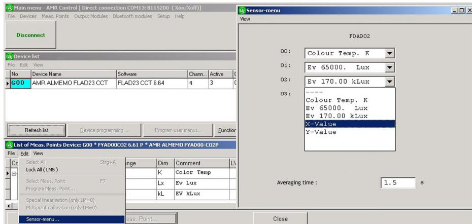
The ranges for the measuring channels can be configured from a list of ranges (\* factory default settings).
