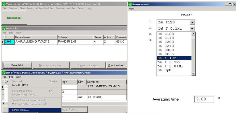
Initially, depending on the rotating vane type, only 1 measuring range is programmed (\* factory default settings). However, if so required, this range can be changed and additional ranges for frequency and rpm can also be configured on the 4 measuring channels.
